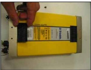
To correctly position the Velcro in the lid of the TrueTracker box, partially attach the two provided mating pieces of Velcro to the receiver, remove the protective film and place the receiver in the box as shown. The adhesive on the Velcro sticks to the cover of the TrueTracker box.
