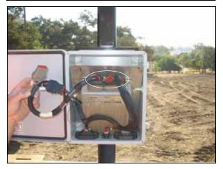
Attach the controller to the aluminum mounting plate with the connectors pointing up. Use 10-32 screws.
