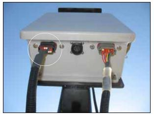
Attach the steering valve harness extension to the existing steering valve connectors and then route the cable to the steering valve.
