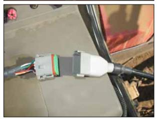
Attach the Sonalert to the extension on the cab interconnect cable.
