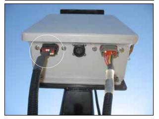
Attach the Steering valve harness extension to the existing steering valve connectors.
