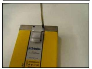
Stick the provided high-strength Velcro to the receiver in the position shown.
