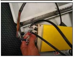
Place the receiver in the cover of the TrueTracker box and then press firmly to fix the receiver to the Velcro.
