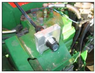
• Weld the provided bar stock to the tractor and then attach the bulkhead to the bar stock.
