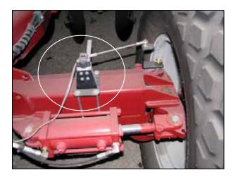
Connect the implement extension cable to the round bulkhead connector at the controller.
