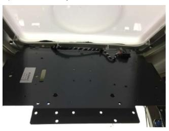
2. Remove the antenna mounting tray. Center the guidance controller on the tray.
