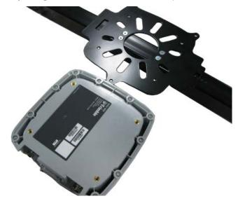
4. Lay the mounting plate with spar attached over on top. Attach the plate to the guidance controller with the four 6 mm bolts and lock washers. Tighten the bolts. Take care not to over-tighten the bolts as damage may result.
