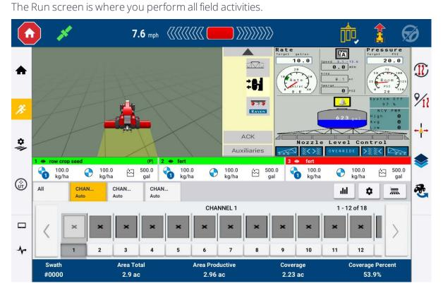
While in the Run screen, Precision-IQ records all field activity (vehicle performance, material application, field coverage, etc.). Data collected can be transferred to your office where your farm is managed.
