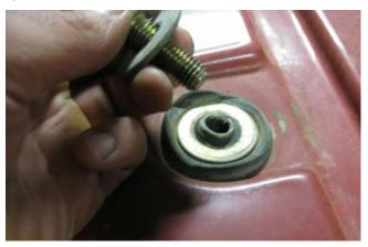
6. Place the supplied spacer on the cab mounting point. The thickness of the spacer will vary by kit.
