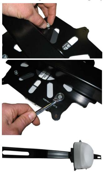
5. Loosen and remove the large bolts on the cab that are to be used to fasten down the spar.
