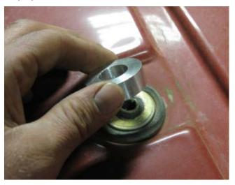
7. Locate the provided longer bolts to be use for securing the spar. Put both the original washer and the larger provided washer on the bolt.
