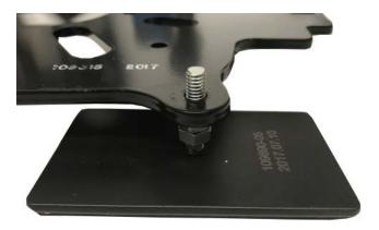
3. Place the flat washer and lock washer on the stud. Loosely thread the remaining nut onto the stud.
