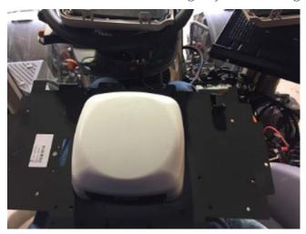
3. Use the base mounting plate as a template to mark and drill ¼" holes for mounting the guidance controller.
