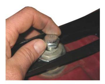
9. Insert the bolt on the other side of the cab. Center the spar on the cab using a measuring tape. Then tighten the bolts.
