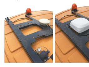
2. Insert, twist, and latch the opposite side of the plate.
