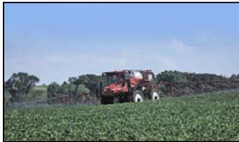
When controlled with the Multi-Application Control plugin, the sprayer can control up to 4 products at once.
