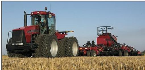
When controlled with the Multi-Application Control plugin, the air seeder can support up to 4 channels of material at once, enabling you to plant combinations of seed or to plant the seeds with liquid, granular fertilizer, or anhydrous ammonia.
