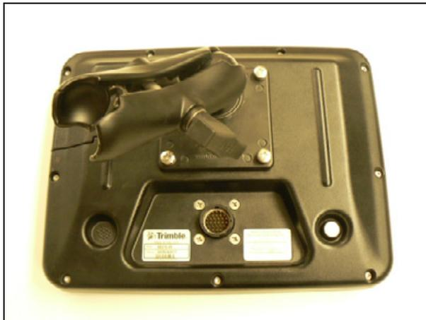
3. Select where in the cab you would like the display to be. The AgGPS FieldManager display is mounted in the cab with a bar style RAM mount.
