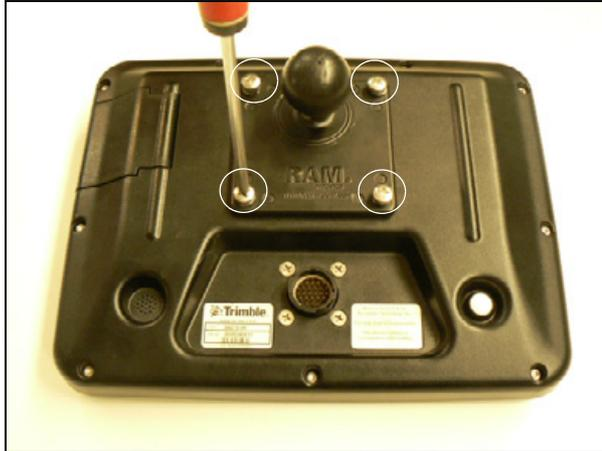
2. Attach the RAM mount to the ball on the mounting plate.
