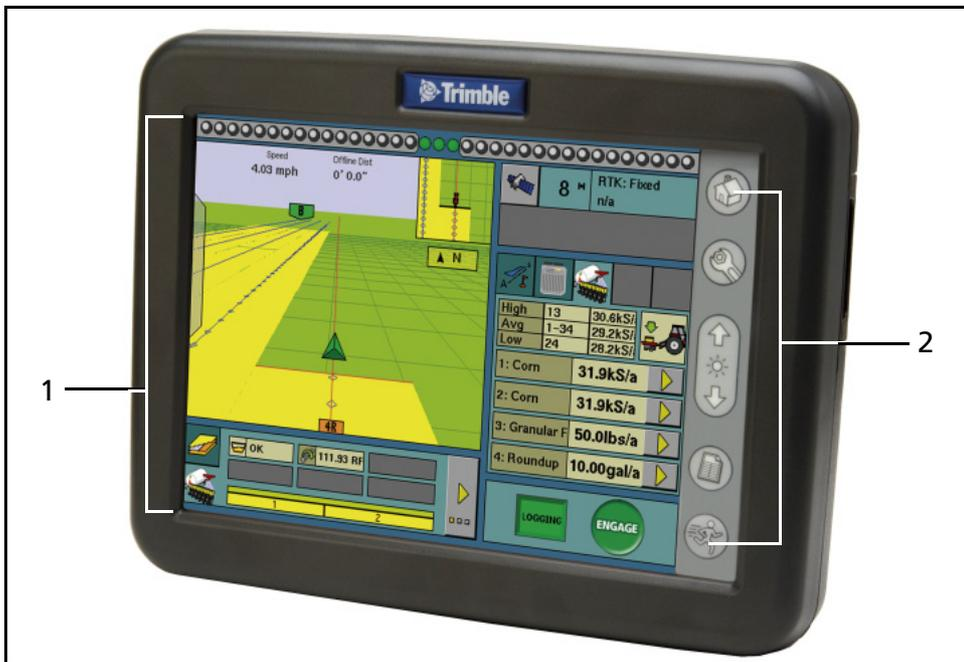
Figure 2.2 The front of the AgGPS FieldManager display unit
