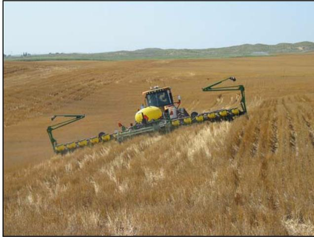
Figure 11.1 Vehicle with implement on a slope
