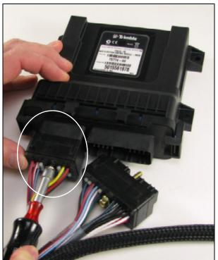
Use a ¼" socket or nut driver to connect the 30-pin connector on the adapter cable to the Rate and Section Control module.
