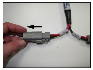
Locate and connect the 4-pin Deutsch DTP receptacle on the FmX integrated display power adapter to the 4-pin Deutsch DTP plug on the power bus.
