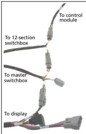
2. Mount and connect the Rate and Section Control module:
