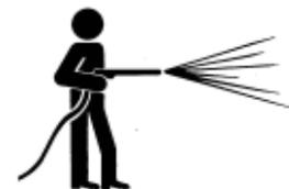
Set the hose pressure as low as practicable, and spray at a 45° to 90° angle. Keep the nozzle of the power washer away from the machine at the distance recommended by the manufacturer.
